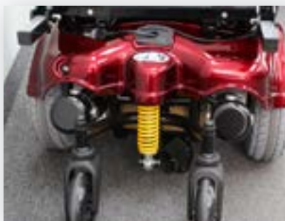
Adjustable Rear Suspension
