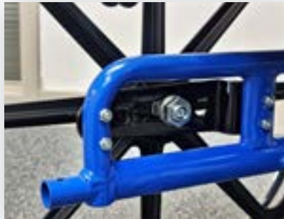
Rear Axle Adjustability Maximizing Hand to Wheel Contact
