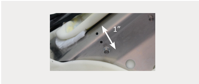
Reposition pin hardware back by 1" on the shell. Optional 1" longer pins to mount a smaller back on a wider chair
