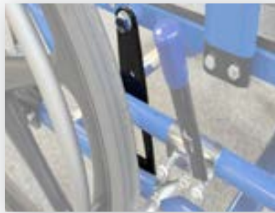
Upper Frame Back Cane, and Front Rigging Adjustable to Balance Center of Gravity
