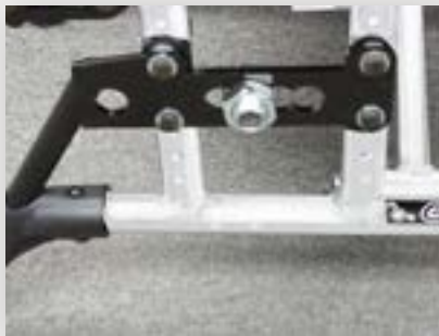
Horizontal Rear Axle Adjustability Ranging From 12.5" To 18.25"
